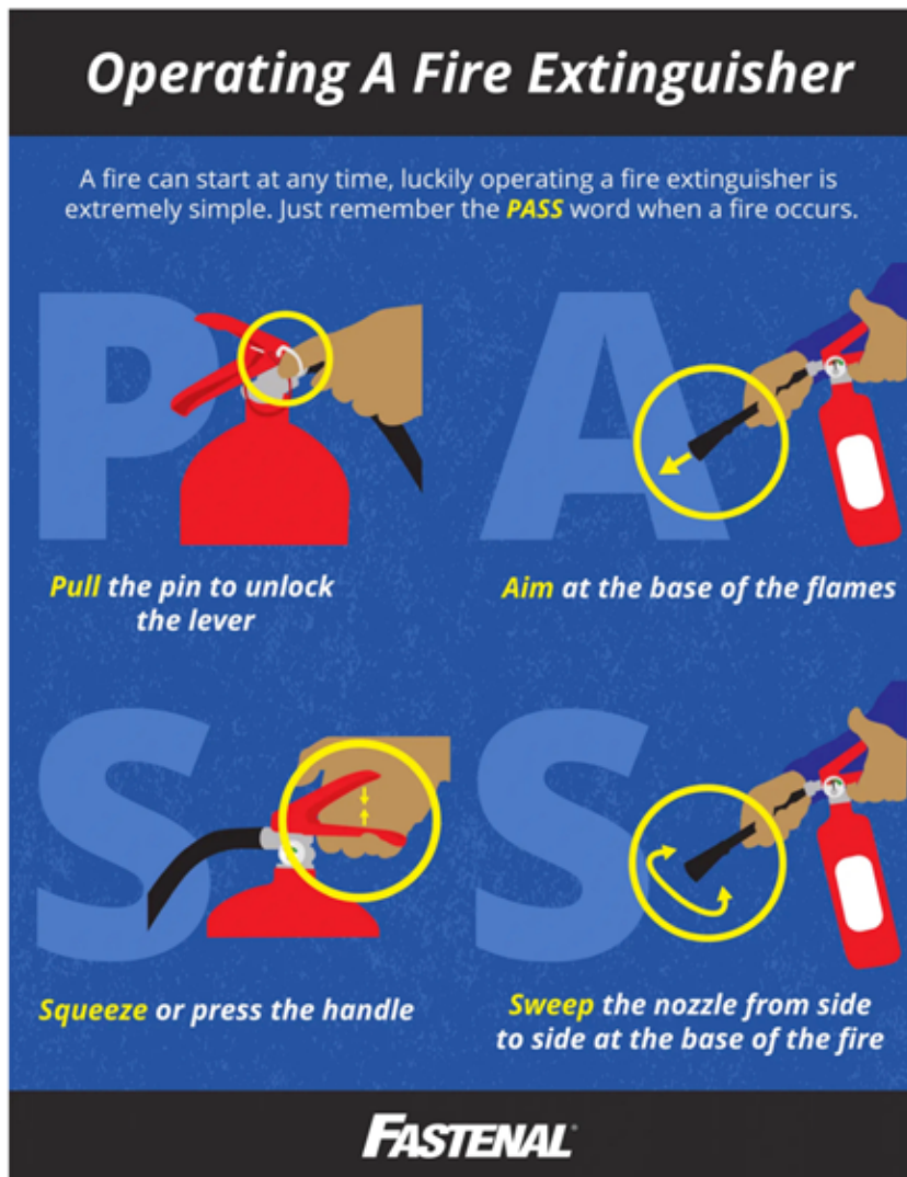
Proper usage of fire extinguisher
