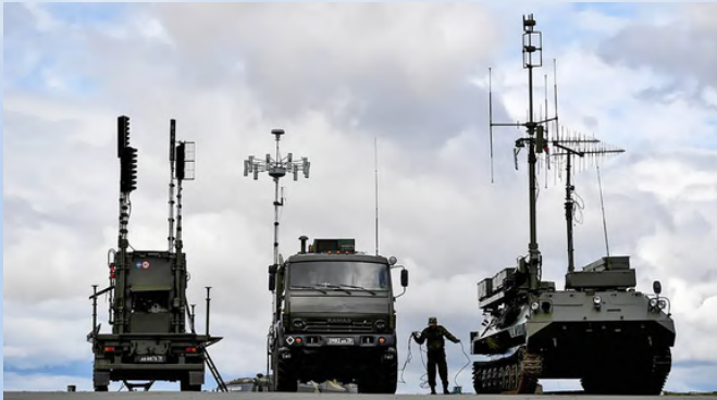
Russia's Krasukha-4 Electronic Warfare System positioned near Ukrainian border, designed to jam enemy radar and satellite signals. Photo Credit: The Warzone (twz.com)
