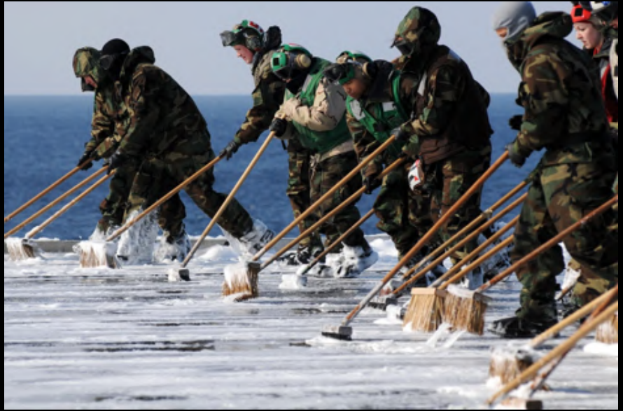
▲ Sailors scrub the flight deck aboard the aircraft carrier, a counter measure wash down to decontaminate the flight deck while the ship is operating off the coast of Japan to remove potential radiation contamination. – Source: Defense Visual Info Distribution Service.
